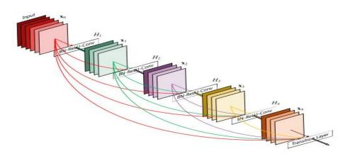
Figure 8 – DenseNet Model Architecture [12]
