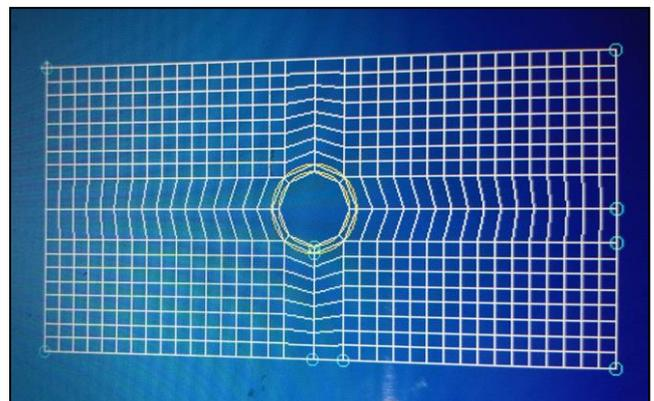
Fig-3: Mirror meshed stiffened panel and cut-out
