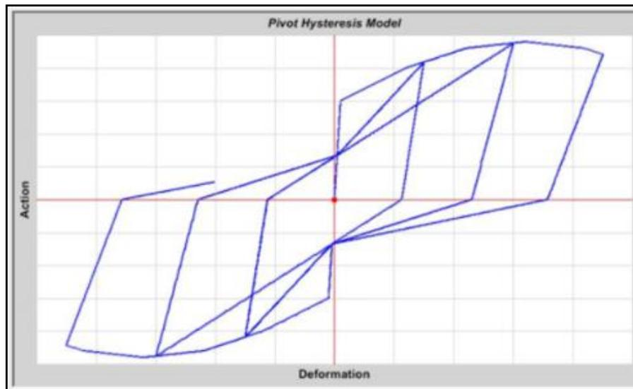
Figure.1 Hysteresis behaviour of SMA bracing
