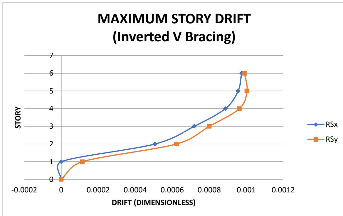
Figure.6 Maximum Story Drift (Inverted V Bracing)
