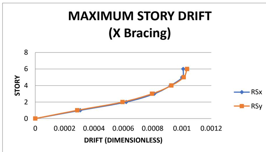
Figure.5 Maximum Story Drift (X-Bracing)
