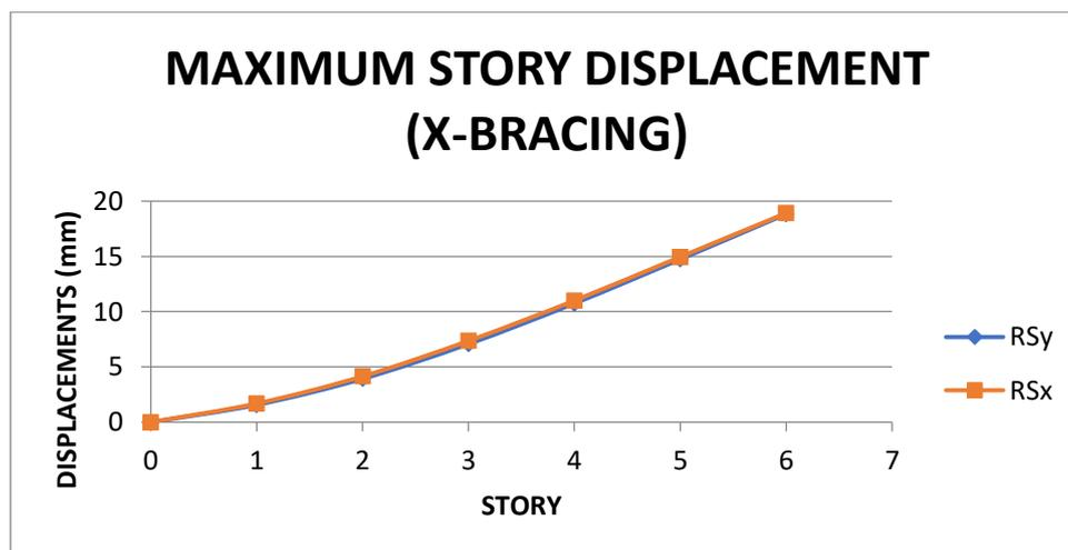
Figure.7 Maximum Story Displacements (X-Bracing)
