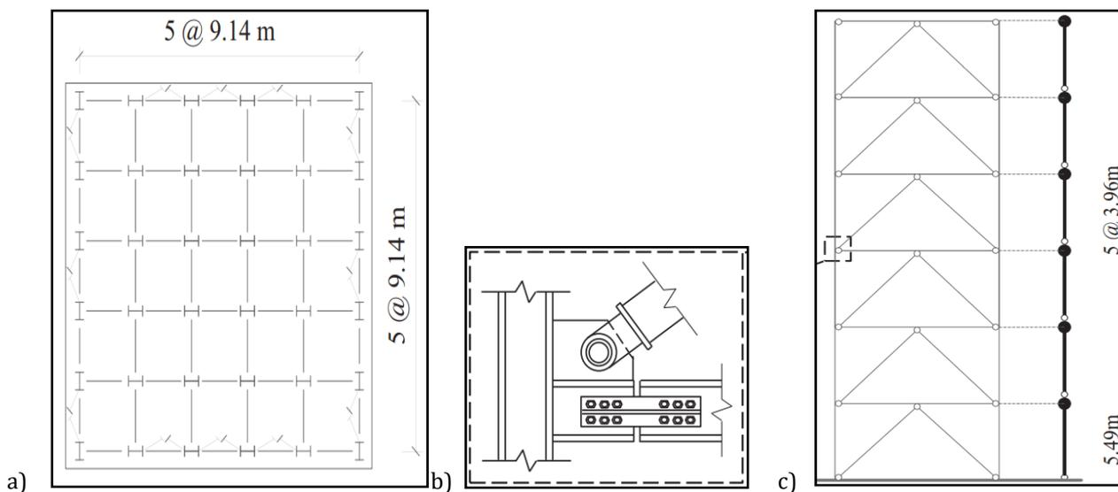
Figure 3. 6-story frame building with SMAB: (a) plan layout; (b) beam-bracing-column connections;
