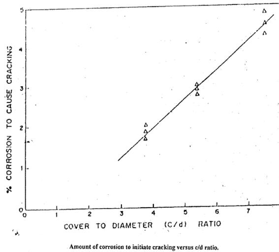
**Fig 4 Amount of corrosion to initiate cracking versus C/D ratio**
