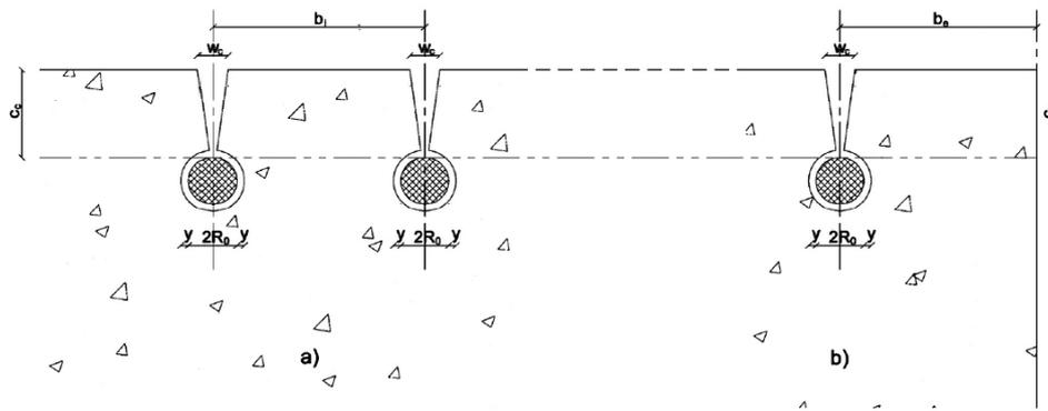
geometric parameters of FEM analyses: a) internal bar, b) external bar
