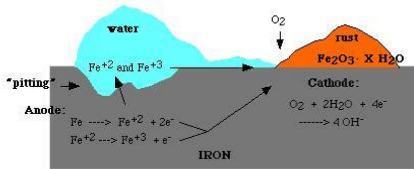
Fig 2 Corrosion process
