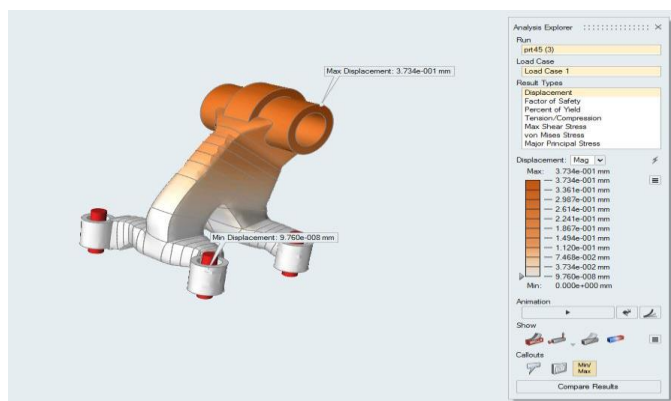
Fig -17: displacement of optimized model
