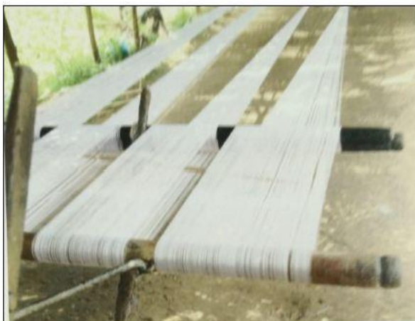
Fig.10.Sizing and starching of fibre.
