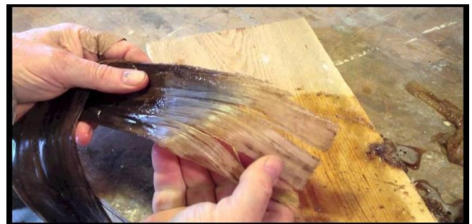
Fig.4. Scraping the Banana pseudo-stem.
