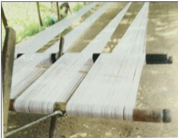
Fig. 9. Brushing the yarn before starching .
