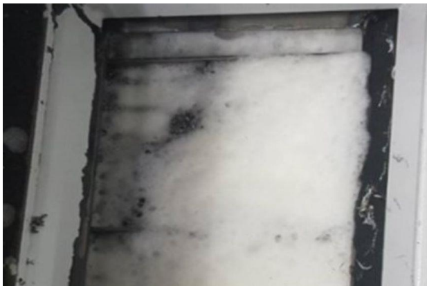
Fig 9. Foaming of coolant
