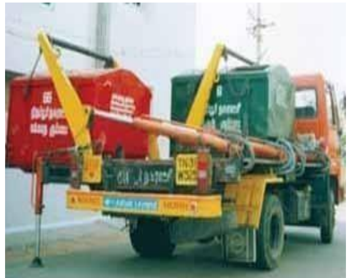
Fig -3: Skip Truck (Dumper placer machines)
