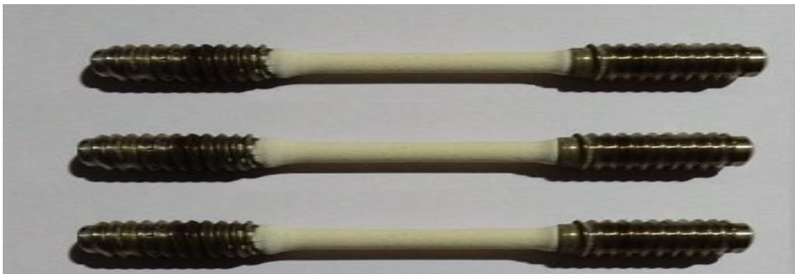
Figure 4: 300 microns AISI 316L specimens just sprayed with the coating powder.
