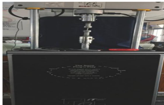
Fig -2: Specimen mounted on the Plug-N-Play Fatigue Testing Machine
