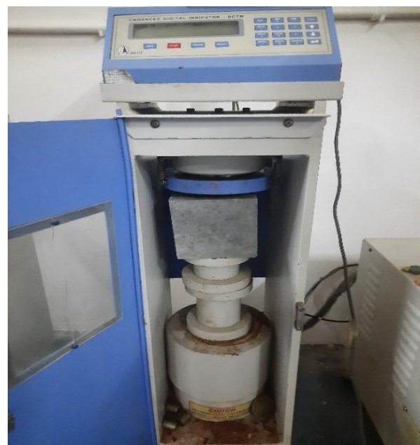
Figure 3: compressive strength test machine.
