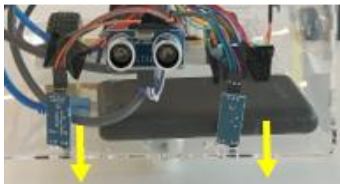
Fig-5: IR Sensors detecting line
