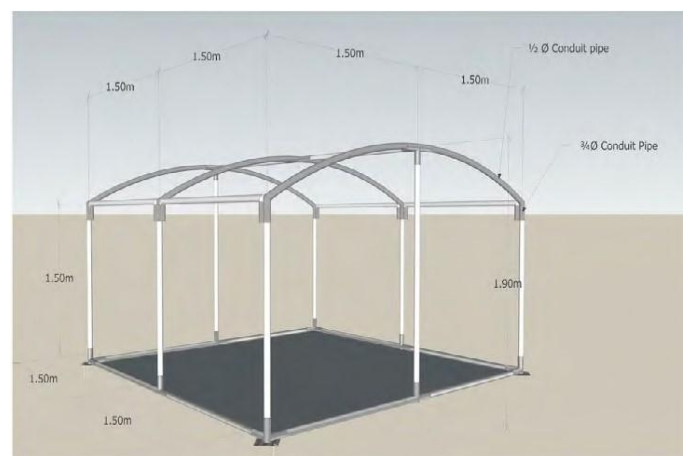
Fig -1: Perspective of Temporary framing
