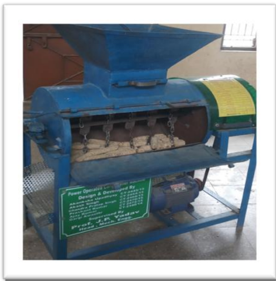
Fig -1: Shelling Tool (having chain spikes)
