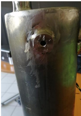
Fig- 2 Placement of thermowells.
