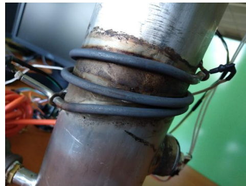
Fig-4 Placement of resistance.
