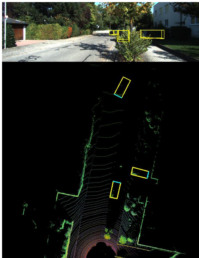
Fig. 7. Model prediction in KITTI [9] test data. The upper part is re projection of the 3D boxes into image space
