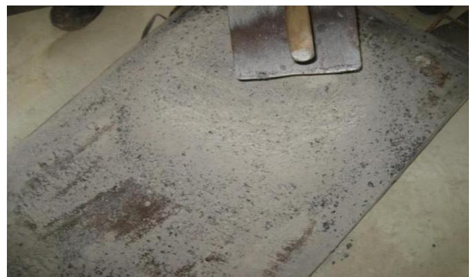
Fig -2: Dry Mixing of Materials
