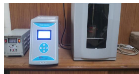
Fig 1 Dispersion of nano clay into epoxy resin using probe sonicator
