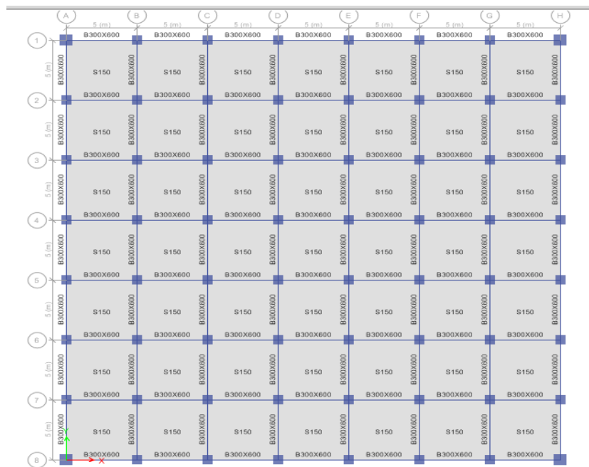
Fig.(3.2) Symmetrical structure plan upto storey 8.
