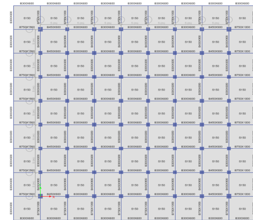
Fig.(3.3) Symmetrical structure plan storey 9 & Above.
