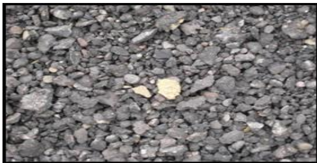
Fig 1 Reclaimed Asphalt Pavement
