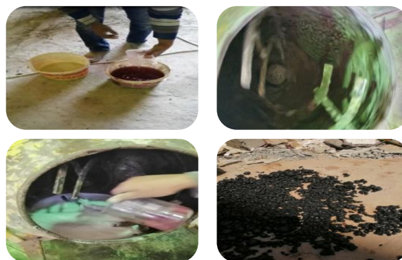
Fig -1: Steps of manufacturing the coarse aggregates
