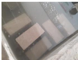
Fig 5.3 Water Absorption test
