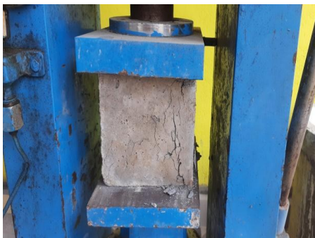
Fig-3 Testing of compressive strength
