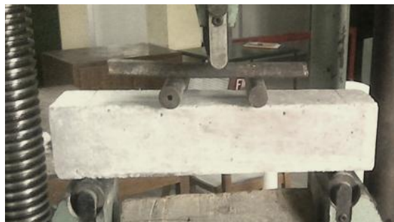
Fig-4 Test set up for modulus of rupture
