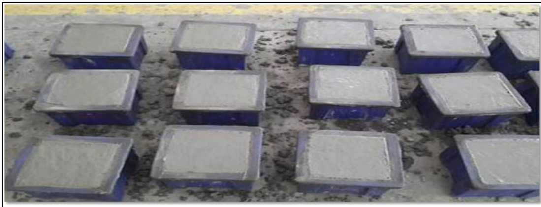
Fig. 1. Casting of concrete blocks
