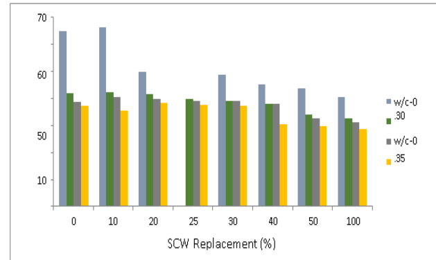
Figure 6 Compressive Strength Values versus SCW replacement (28-days)
