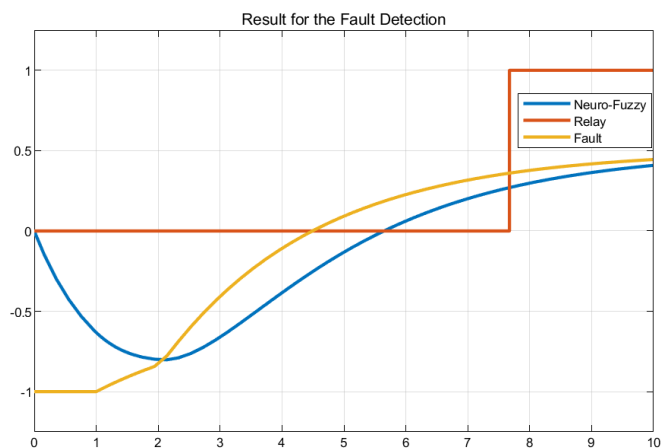
Fig -15: Results for the detection of fault using Neuro-fuzzy controller.
