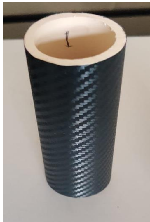
Fig -1 Woven carbon fiber matt on CPVC pipe
