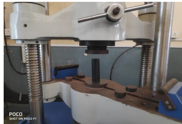
Fig-4 Compression test on Reinforced tube
