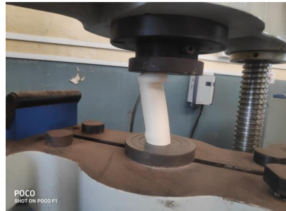
Fig-3 Compression test on non-reinforced tube
