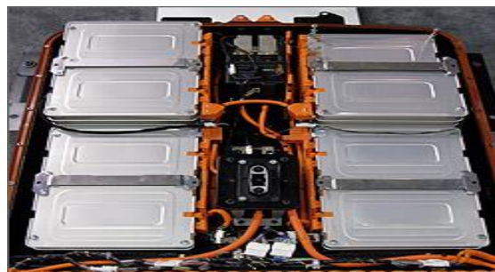
Fig 5: A typical example of LI-ion batteries used in EVs
