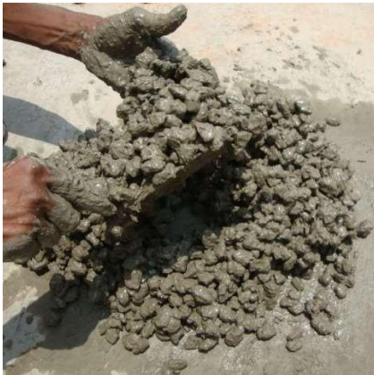
Fig 2 Crushed Over Burnt Bricks
