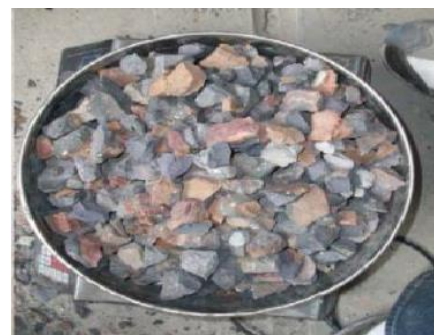
Fig 1 Crushed Over Burnt Bricks
