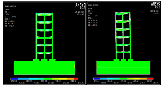
Fig.-25 : Stress in X direction of Model-5& Model 6
