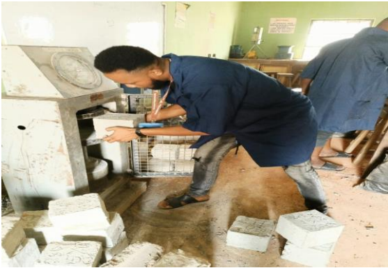
Figure 2. Crushing of Concrete Cubes
