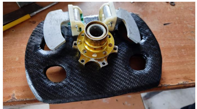
Fig -6: Manufactured Assembly of Steering wheel with paddles.
