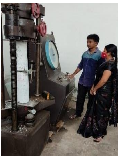
Figure 6: Testing of Column in UTM
