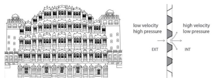
Fig -6: Sketches showing the windows to wall ratio and the wind flow
