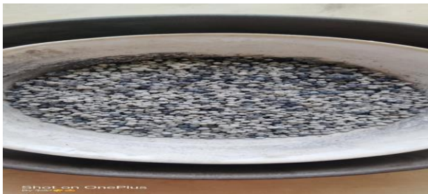
Fig 2.2. ZnO catalyst coated on glass beads
