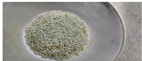
Fig 2.1. TiO 2 catalyst coated on glass beads
