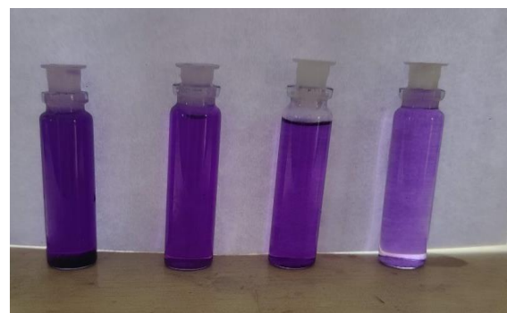
Fig.5.6. Degradation of Crystal Violet with Catalyst ZnO
