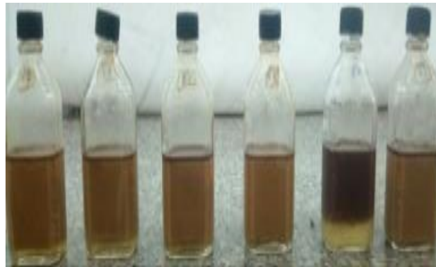
Figure 34: Emulsion treatment using Grape demulsifier
