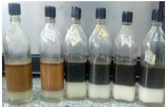
Figure 31: Emulsion treatment with Servo demulsifier
