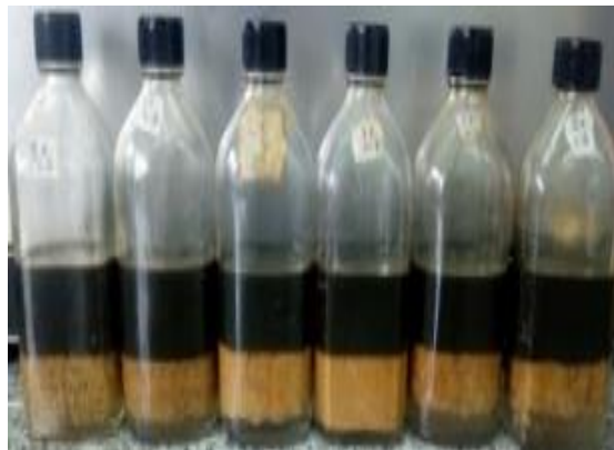
Figure 32: Emulsion treatment with Separol demulsifier
