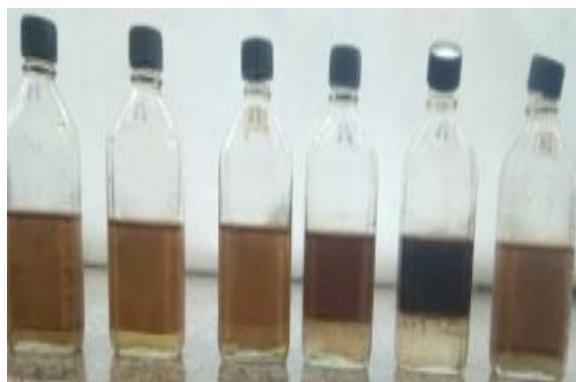
Figure 33: Emulsion treatment using Lime demulsifier
