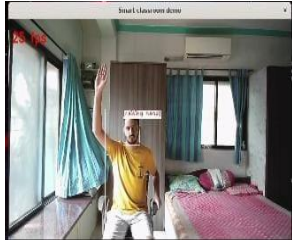
Fig -6: Smart classroom action recognition and face detection implementation
