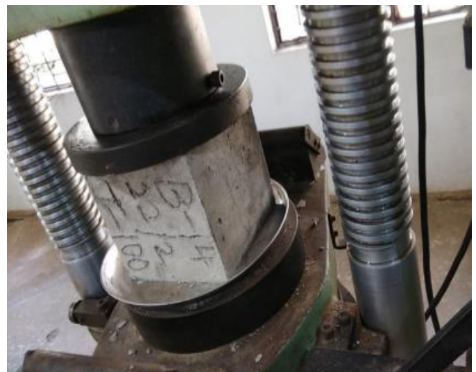
Fig -6: Compressive Testing for Sample of Cube
