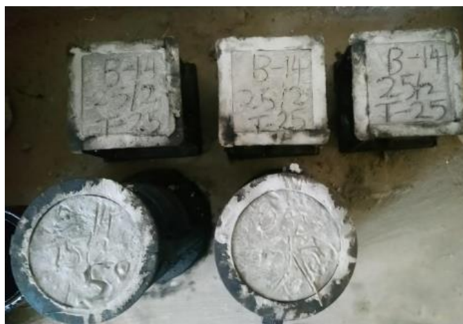
Fig -4: Casting of Cubes & Cylinders
