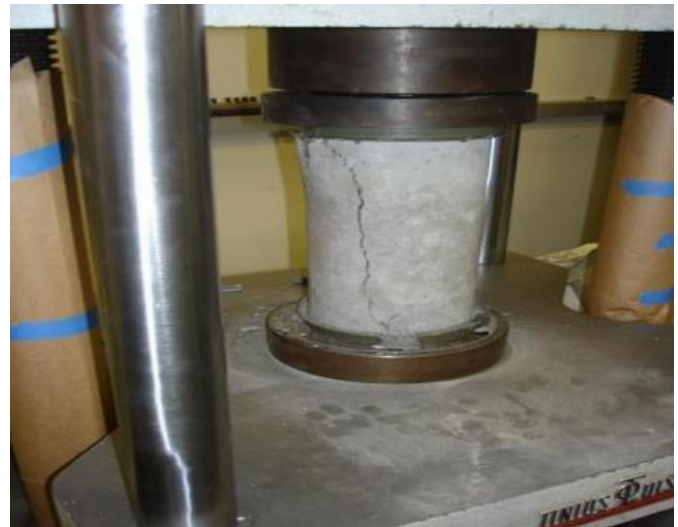
Fig -5: Compressive Testing for Sample of Cylinder
