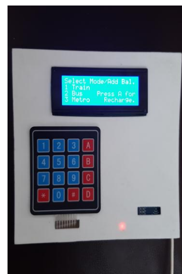
Fig -4: Hardware system enclosed in a 3D printed enclosure
