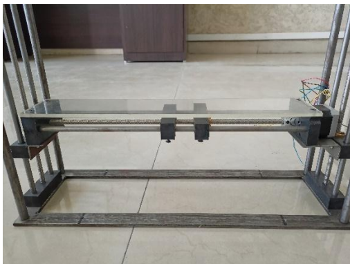
Figure 12- Structure for x-axis operation
