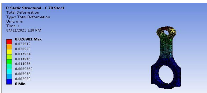
Fig. 7: Details of Deformation in Steel material
