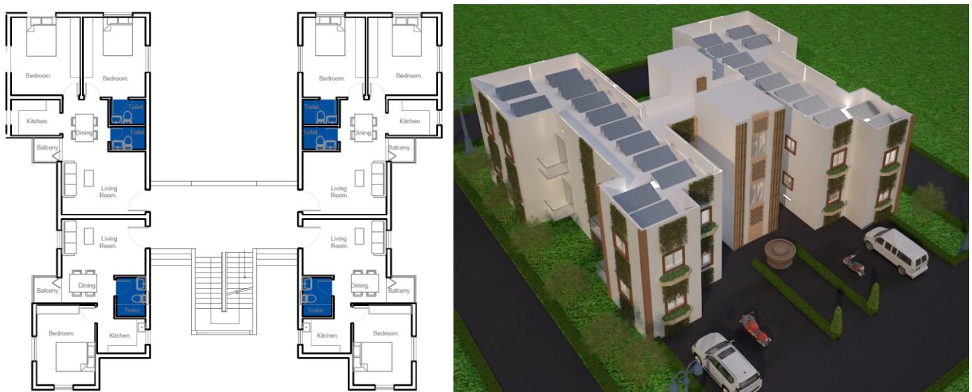
Figure 2 Shows Layout drawing & 3D Model of GFRG Building By Using Autocad & Revit
