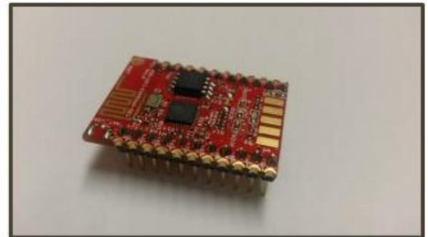
Figure 3.8 Olimex MOD-WIFI-ESP8266-DEV module used in this thesis
