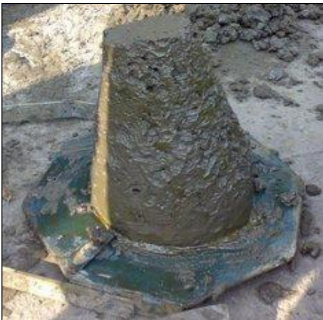
Fig -3: Slump cone test
