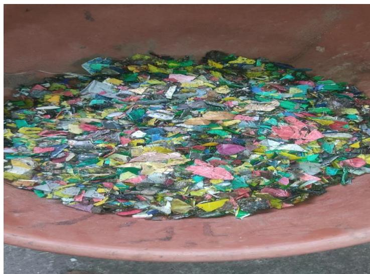
Fig no 1.2 High Density Polyethylene waste plastic crush (HDPE)
