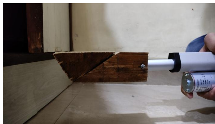
Fig -4: Locking Mechanism (Unlocked)
