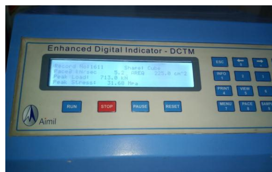
Fig -8: CTM Reading.
