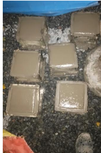
Fig -3: Cube Casting.
