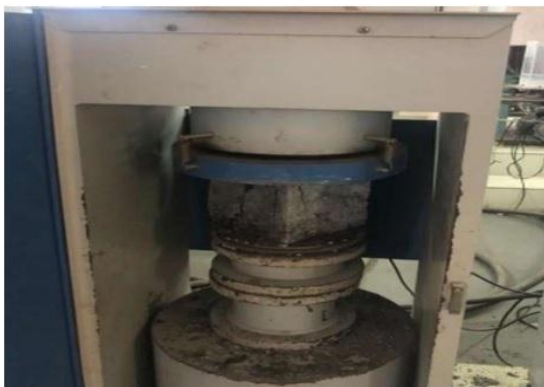
Fig -1: Cube Testing
