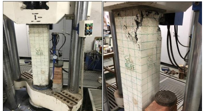
Fig -6: Testing on column with HDPE pipe
