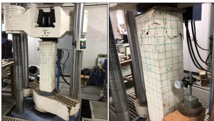
Fig -4: Testing on column without pipe
