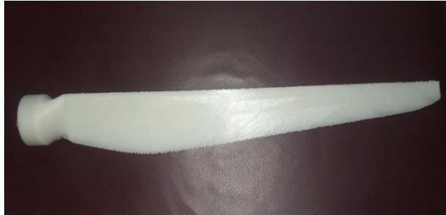
Fig. 3:3D Printed Wind turbine Blade
