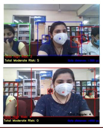
The Output displays all the pedestrians detected and highlighted with their Class IDs and therefore the confidence corresponding to detections. Also, every case in violation of social distancing i.e., when distance in pixelsis over the configured one, ishigh lighted in an exceedingly red color bounding box. The Total Number of violations detected is displayed at the bottom of the frame.
