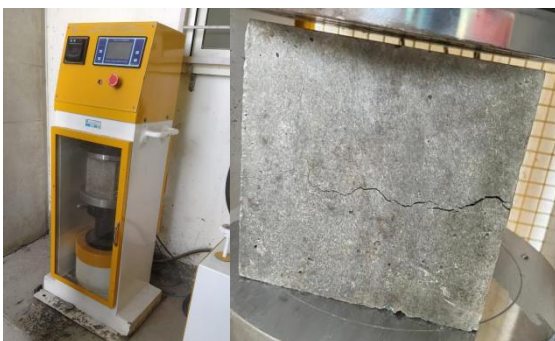
Fig.3 compressive test on concrete cube of bacillus megaterium de Bary (ATCC 14581)
