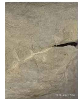
Fig 4(b) 75% healed crack
